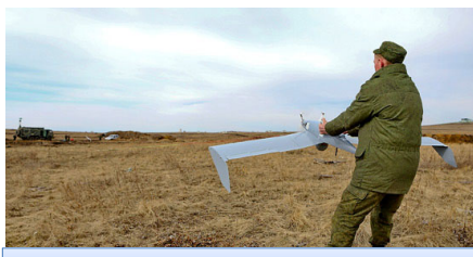
Launching UAV with a rubber catapult. Photo from the official site of Ministry of Defense of RF http://mil.ru/924gcba/equipment
