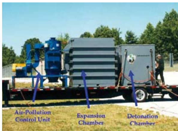
Figure 4.6: Mobile version of detonation chamber with expansion and air pollution control unit
