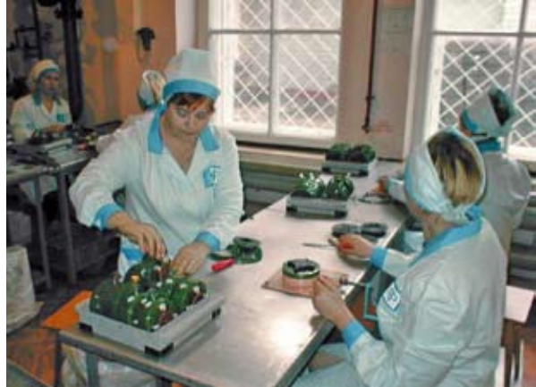
Fig. 5.1: Manual disassembly of anti-personnel landmines (Donetsk, Ukraine)
