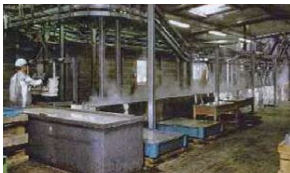
Figure 6.2: Recovery of white phosphorus using melt out
