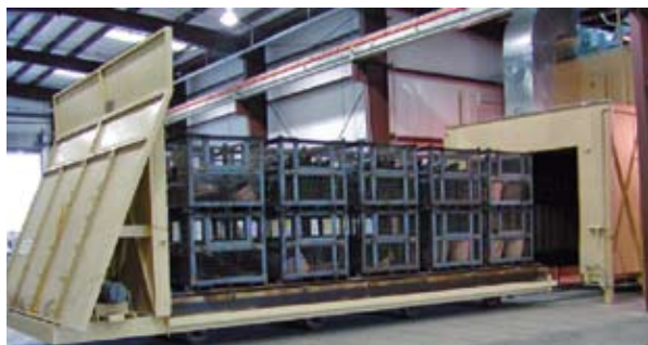
Figure 4.5: Hot gas decontamination facility. The rail car is charged with metal baskets that are loaded with pre-treated ammunition.
