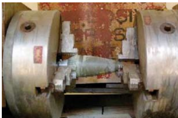
Figure 5.2: Lathe for the cutting of 81 mm mortar
