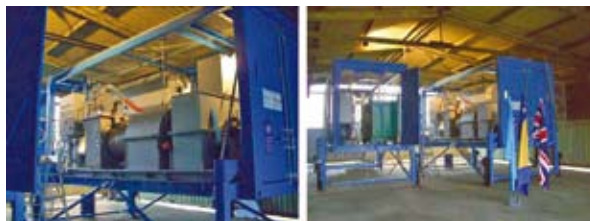
Figure 4.2: Containerized Ammunition Destruction System as used by Bosnia UNDP
