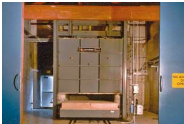
Figure 4.4: Car bottom furnace with door half open
