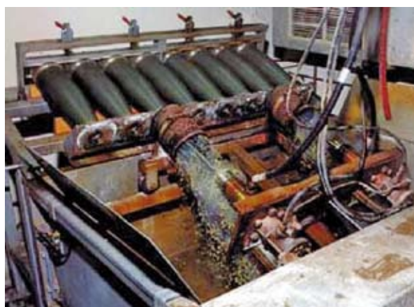
Figure 6.3: Water jet washout of 155 mm shells
