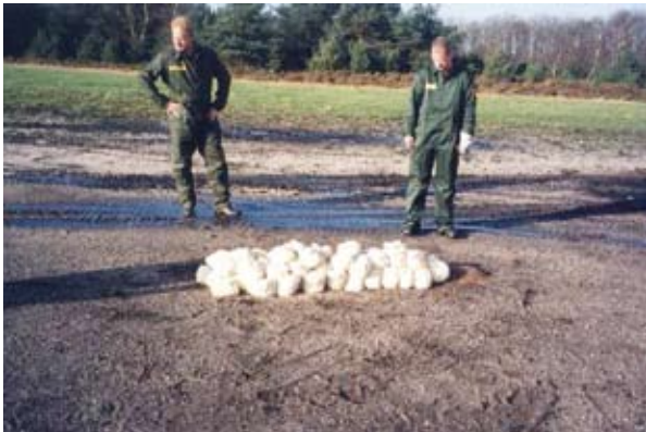
Figure 3.2: Bags filled with propellant, ready for open burning
