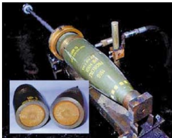
Figure 5.3: Equipment for hydro abrasive cutting, insert picture 155 mm cutting result
